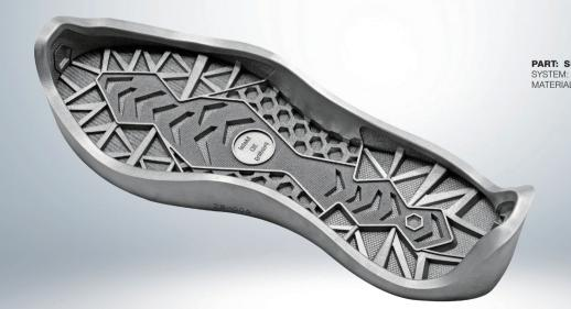
PART: SHOE MOLD SYSTEM: FS200M-2 MATERIAL: 316L
